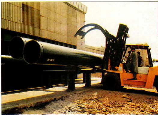
*Precoated pipes from the outgoing racks being transferred to storage area.*
