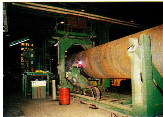
*Pipe being cut automatically at the plasma arc cutting station.*
